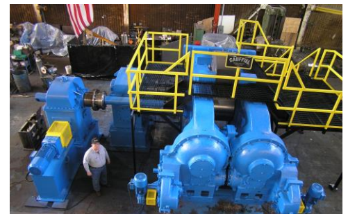
Rolling Mill for Powdered Metal to Any Alloy Strip
