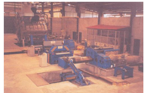
Rolling Mill for Continuous Casting
