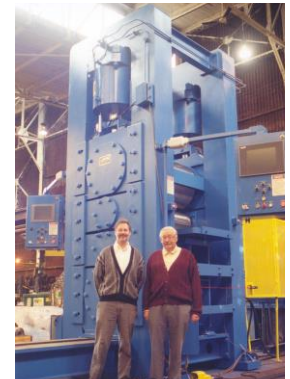
4-High Mill with 2,000,000# of Separating Force
