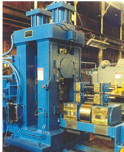
4-High Mill for High Strength Alloys
