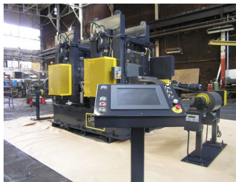
Precision Tandem Mill for Reducing to .001" Thick
