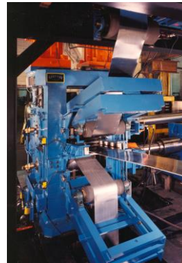
Three-Ply Cladding for Three Layers of Strip
