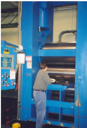
Rolling Mill for Large Computer Targets
