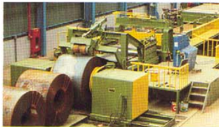
Left, 72" x 3/8" x 60,000 lb. coil capacity Cauffiel pickle line.
