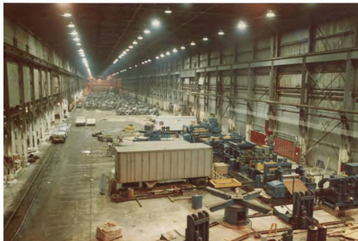
80,000# ABOVE FLOOR COIL PROCESSING LINE IN STEEL MILL FOR INSPECTION AND TENSION LEVELING FOR SPEEDS UP TO 1,000 FPM
