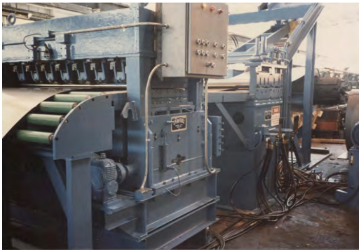
BACKED UP CORRECTIVE LEVELER W/LOOP CONTROL FOR PRESS FEED LINE OR CUT-TO-LENGTH LINE
