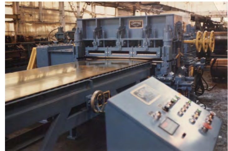
WIDE ROLL BACKED UP CORRECTIVE LEVELER FOR ALUMINUM AND STAINLESS STEEL, NO BACK UP ROLL SHADOWS AS COMMON 4-HIGH LEVELERS
