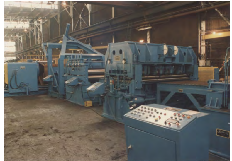
DOUBLE LEVELER CUT-TO-LENGTH LINE READY FOR TESTING UNDER CRANE ON AMERICAN STEEL PRODUCTS' ASSEMBLY AND TESTING FLOOR
