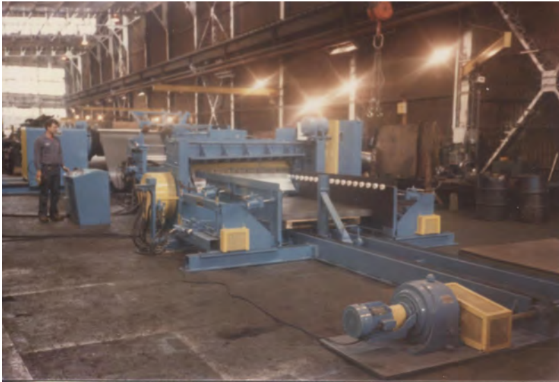
LOOP TYPE, HIGH PRODUCTION CUT-TO-LENGTH LINE, AUTOMATIC STACKER AND FLOOR RUNOUT, WOOD DUNNAGE SHOWN IN STACKER AREA
