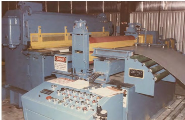
POLYURETHANE ROLL FEED W/LONG EDGE GUIDES AND CANTINEER SECTION FOR STAINLESS STEEL & ALUMINUM FOR CUT-TO-LENGTH OR PRESS FEED LINE
