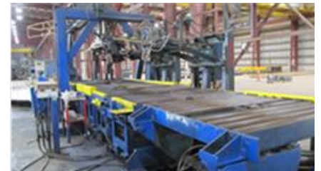
72" x 15,000# Downlayer for Banding Line w/Conveyor System
