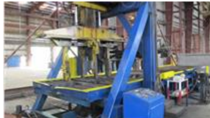
72" OD Automatic Pick & Place Banding System
