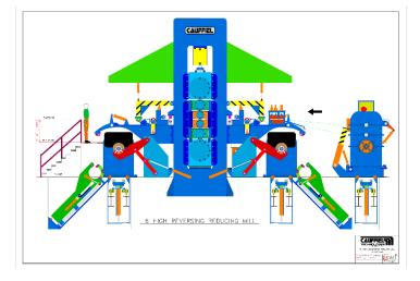
or dual motor driven. Six-high rolling mills are equipped with hydraulic screwdowns, automatic shape control, and automatic gauge control.
