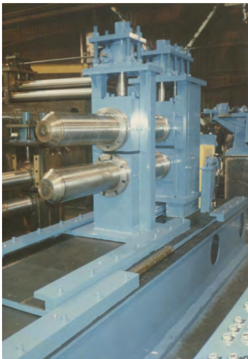
SLITTER W/SLIDING OUTBOARD SUPPORT TO REDUCE SPAN OF ARBORS TO DECREASE DEFLECTION FOR MANY CUTS OF .250" IN SINGLE PASS
