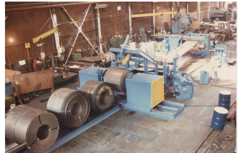
MODERNIZED SLITTING LINE SYSTEM FOR HOT ROLLED STEEL FOR STRUCTURAL TUBE MILL
