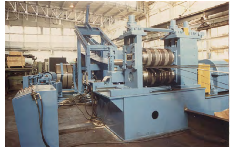
NARROW HEAVY GAUGE SLITTING LINE, 12 CUTS OF .250", ONE PASS, HOT ROLLED STEEL
