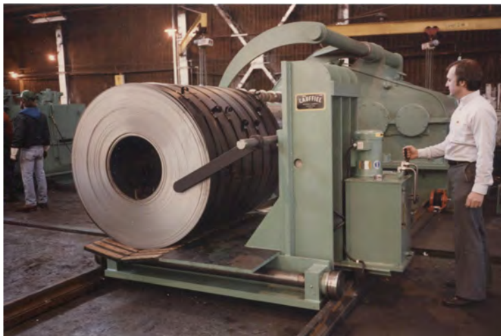
EXIT COIL CAR FROM RECOILER W/HOLDING FINGERS FOR C-HOOK REMOVAL WITHOUT TURNSTILE
