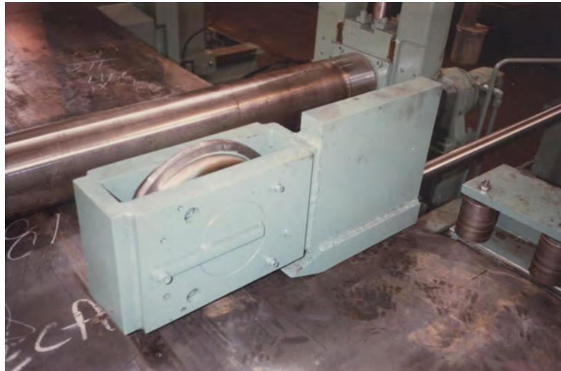
THROATLESS SLITTER TO SLIT MATERIAL FROM 020" TO .500" THICK (REPLACES CROPPING SHEARS IN SLITTING AND ROLL FORMING LINES)
