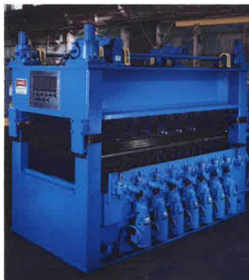
CORRECTIVE LEVELER FOR 72" WIDE X 10 GAUGE
