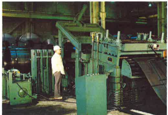
10 GAUGE X 72" X 60,000# PRESS FEED LINE
