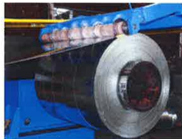
RECONDITIONED SLITTING LINE W/IN LINE CORRECTIVE LEVELER TO ELIMINATE LOOPING PIT
