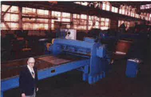
10 GAUGE TO .020" MULTIPLE SLIT BLANKING LINE
