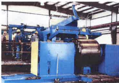
80" X 1/2" X 60,000# SLITTING LINE (UNCOILER SECTION)
