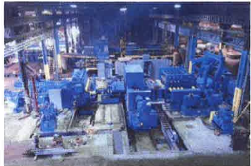
96" X 5/8" X 100,000# DOUBLE LEVELER CUT-TO-LENGTH LINE
