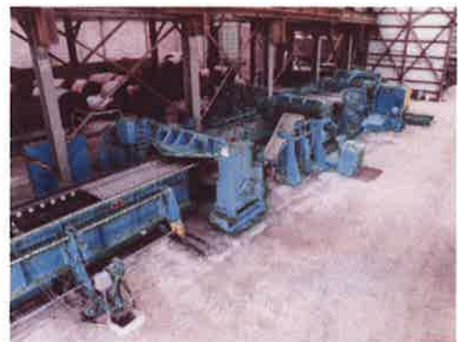
72" X 1/2" TO .020" X 60,000# STOP/GO & LOOP CUT-TO-LENGTH LINE FOR HOT & COLD ROLLED
