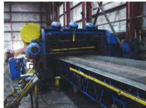
72" X 1/2" TO .062" X 60,000# CUT-TO-LENGTH LINE W/TEMPER MILL
