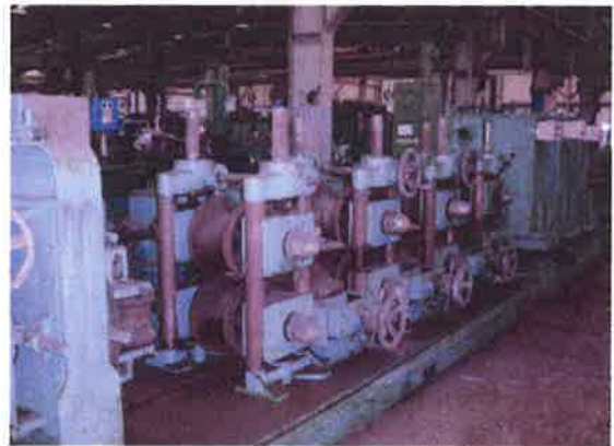
12-1/2" LIGHT WALL STAINLESS STEEL PIPE MILL
