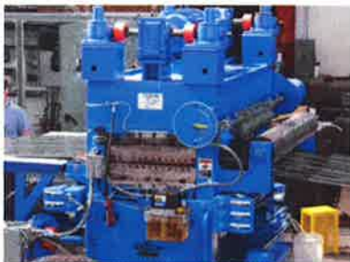
RECONDITIONED SLITTING LINE W/IN LINE CORRECTIVE LEVELER TO ELIMINATE LOOPING PIT
