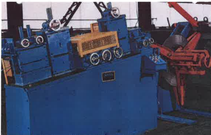
1/4" X 2" HIGH-SPEED LOOP TYPE EDGING LINE W/ROTARY PRESS SHEAR
