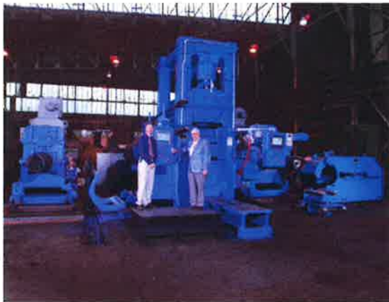
52" WIDE X 1/4" TO .015" THICK 4-HIGH ROLLING MILL W/HYDRAULIC SCREWDOWN
